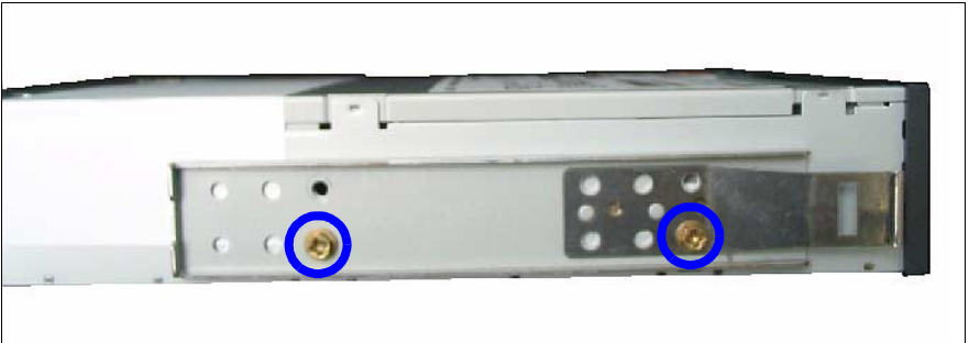
Figure 17: Attaching the EasyClick rails - magnetic tape drive LTO Ultrium 1HH
